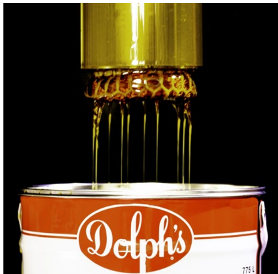
Dipping process for stator impregnation.
