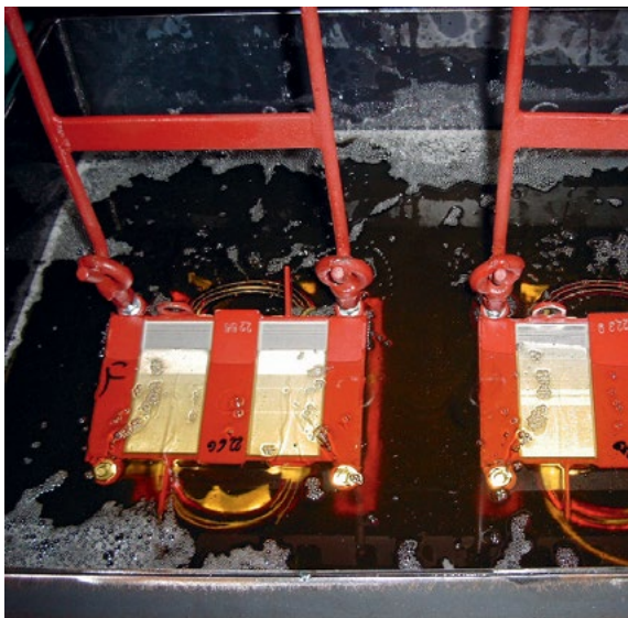
Impregnation dipping of ballasts.
