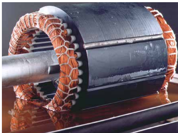
An impregnation resin applied by roll through
